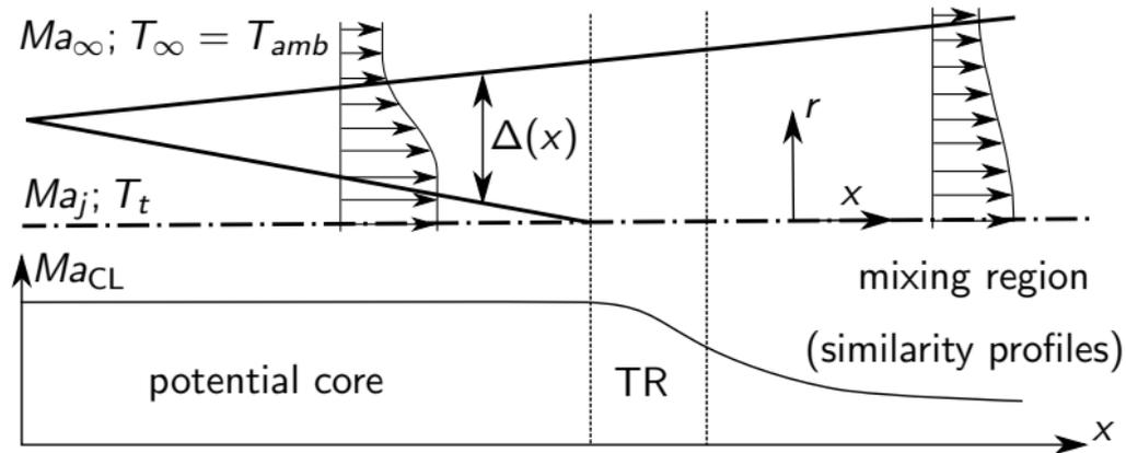
Shear layer growth  $\frac{\partial \Delta}{\partial x}$
