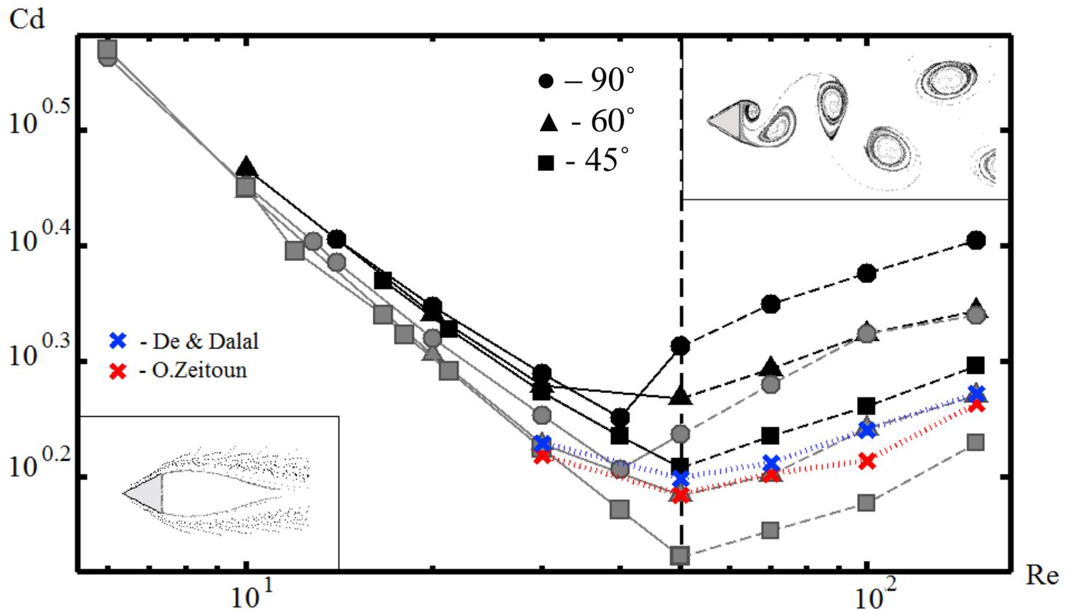
Fig. 2: The drag forces acting on the cylinder. Gray markers – vertex facing flow, black markers – base facing flow.
