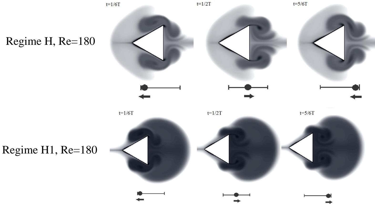
Fig. 5: Flow patterns around vibration-driven robot.
