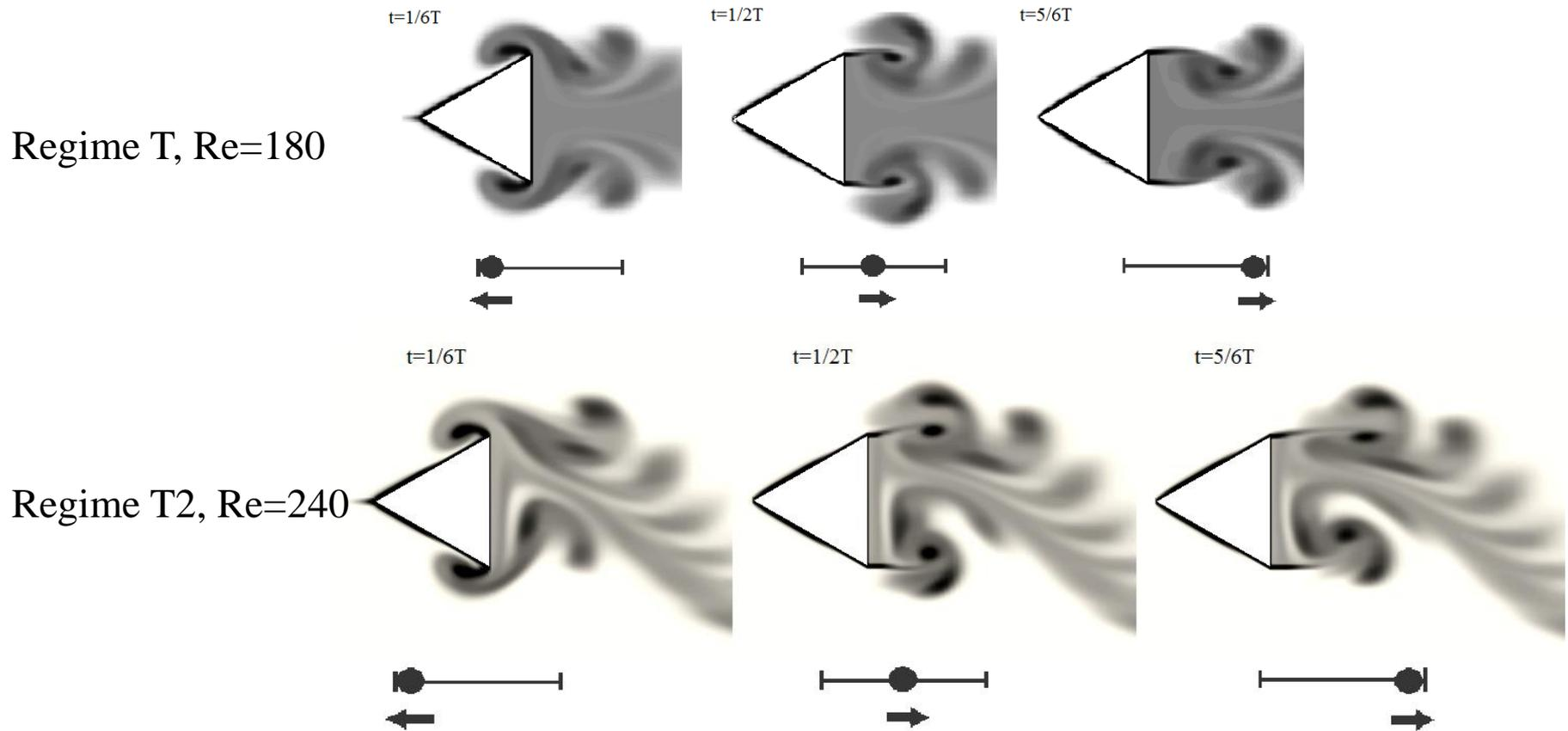
Fig. 7: Flow patterns around vibration-driven robot.
