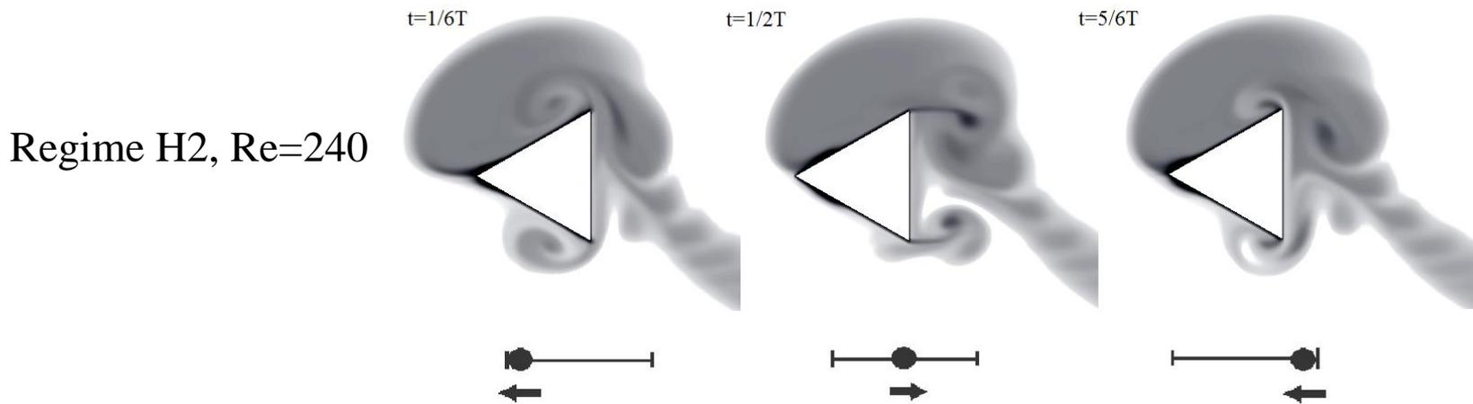
Fig. 6: Flow patterns around vibration-driven robot.
