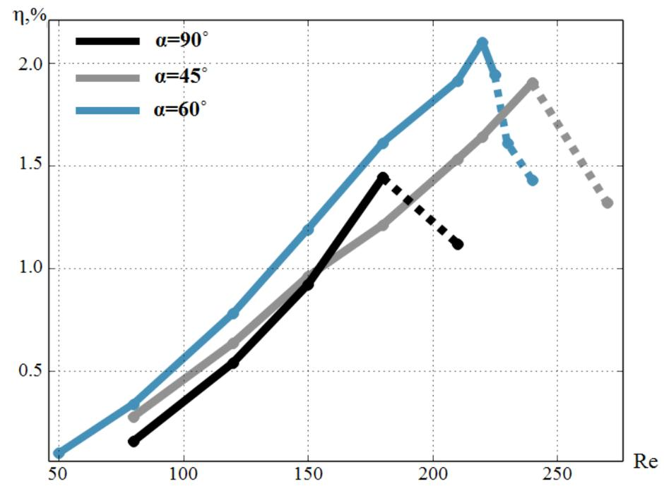
Fig. 9b: Efficiency of movement ( $\eta = \frac{N_0}{N_{vbr}}$ ).
