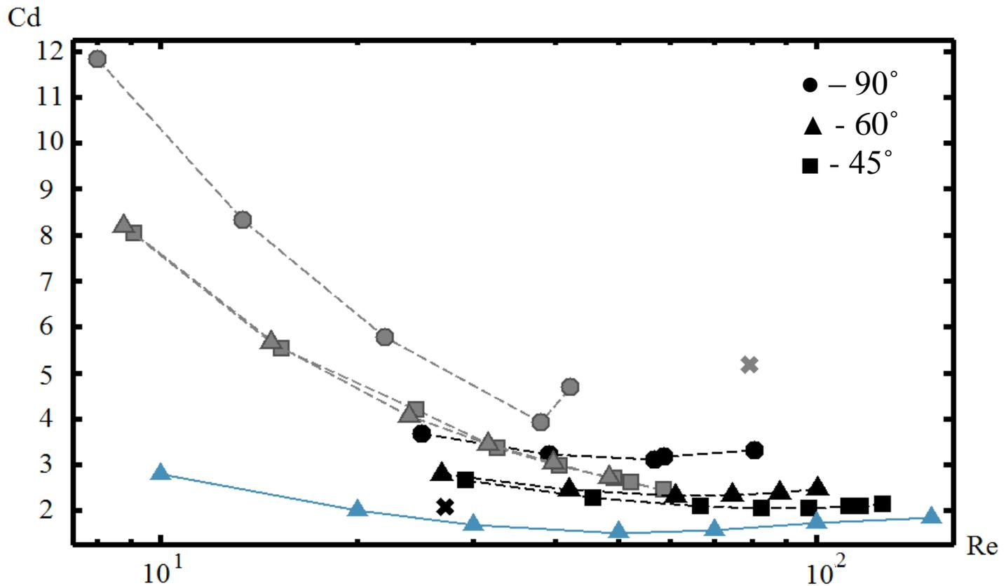
Fig. 11: Drag force coefficients. Gray markers-  $C_{d+}$ , black markers -  $C_{d-}$ . Blue line -  $C_d$  for steady flow past equilateral triangular cylinder.
