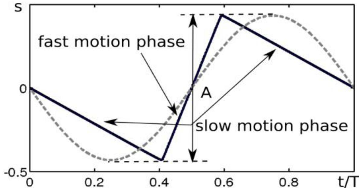
Fig. 4: Harmonic (dashed line) and two-phase\* (solid line) laws of the internal mass motion
