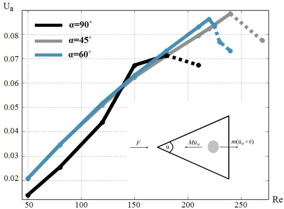
Fig.9a: Average velocity of movement ( $U_a = \langle U \rangle$ )
