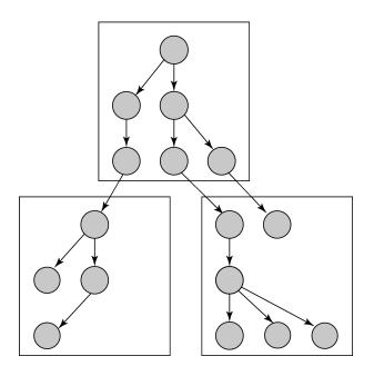
Figure 2: BST block separation example
